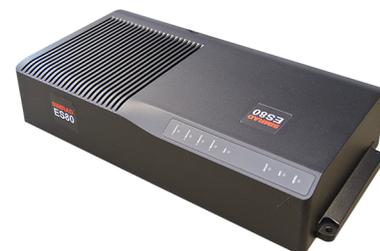
The Wide Band Transceiver (WBT) is designed for applications where performance is the top priority. It has four 500 W channels that can either work independently with single beam transducers, or together with a split beam transducer. The design is optimized for applications where power consumption and physical size is not critical.
