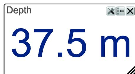
Selecting **Setup** in the *Depth* information pane opens the **Bottom Detection** page in the **Information Pane Options** dialog box. The purpose of the **Bottom Detection** parameters are to define the upper and lower depth limits most likely to be used during the ES80 operation.
